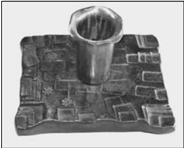
Fly press textured candle holder, candle cup is copper. The tool used to make the deco texture is a used rectangular Whitney punch 3/8" X 5/8" on the business end. I ground the sharp edges slightly. This is one of the first test pieces made with the press.
